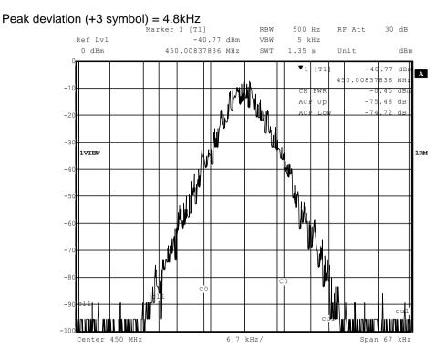
Figure 40 Modulation Spectrum, 25kHz Two-point Mode
