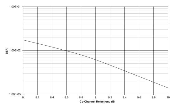
Figure 45 Modem Co-channel Rejection with FM Interferer (as EN 300 113)
