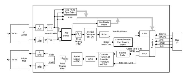
Figure 3 Block Diagram - two-point Tx with I/Q Rx
