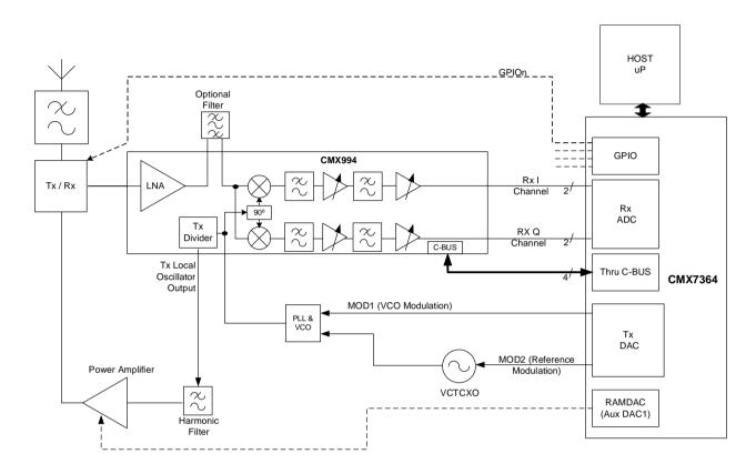
Figure 31 Outline Radio Design (4-FSK - I/Q in, two-point mod out)
