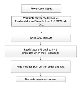
Figure 14 - Reset without FI Load
