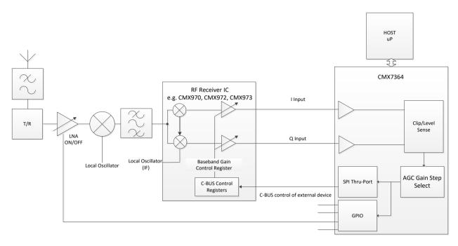
Figure 26 AGC using SPI Thru-Port and external LNA
