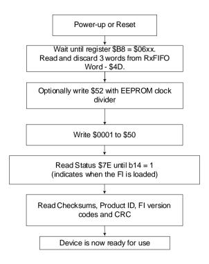
Figure 13 - FI Loading from Serial Memory
