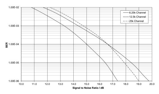
Figure 42 Modem Sensitivity Performance (Root Raised Cosine Pulse Shaping)
