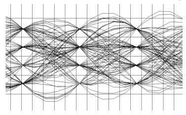
Figure 21 Received Eye Diagram
