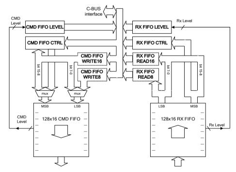
Figure 24 Command and Rx Data FIFOs
