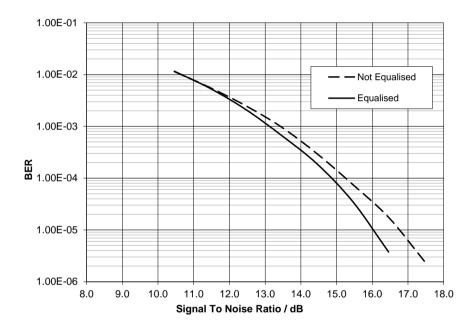
Figure 47 4-FSK Signal-to-Noise Performance, Equalised and Non-Equalised
