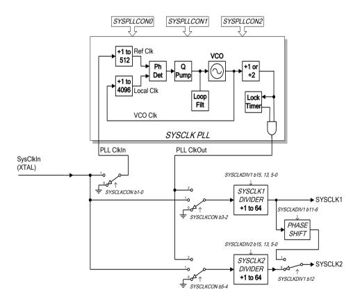
Figure 29 Digital System Clock Generation Schemes
