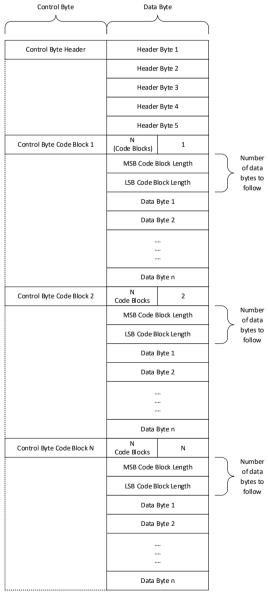
Figure 32 Received RTCM SC135 Frame
