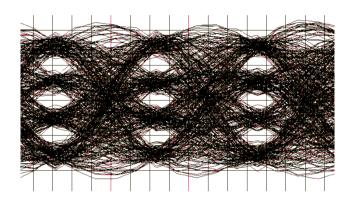
Figure 20 Transmit Eye Diagram
