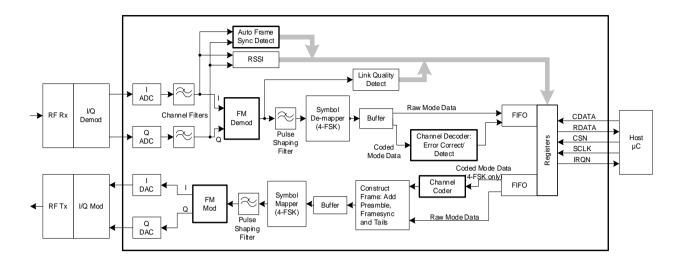
Figure 2 Block Diagram - I/Q Tx and Rx
