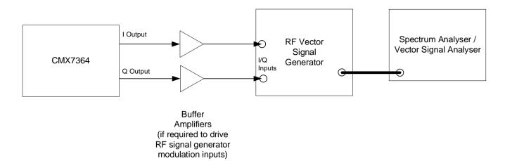
Figure 33 Tx Spectrum and Modulation Measurement Configuration for I/Q Operation
