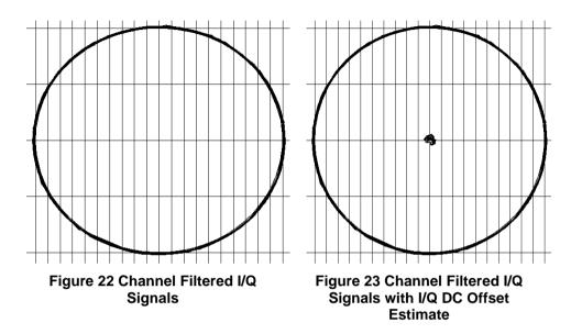
**Note:** The images of receive diagnostic modes shown above are idealised. In practice when using the I Output and Q Output signals to view diagnostics the transitions between constellation point are not instantaneous. Using an analogue oscilloscope is the best way to observe these diagnostic signals.
