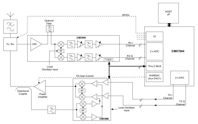
Figure 30 Outline Radio Design (I/Q in/out)
