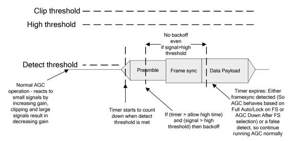
Figure 27 AGC Behaviour During Burst Reception
