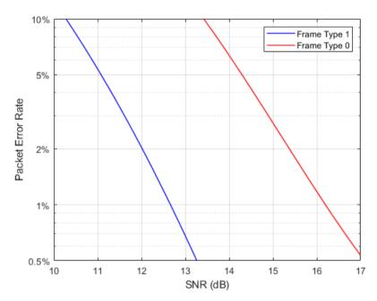
Figure 44 RTCM Header Packet Error Rate: 12.5kHz Channel, 4.8ksymbols/s
