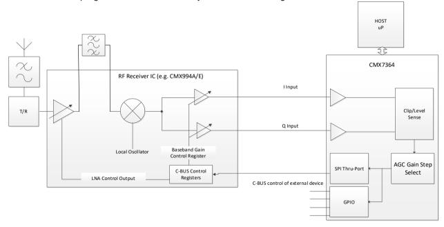
Figure 25 AGC using SPI Thru-Port
