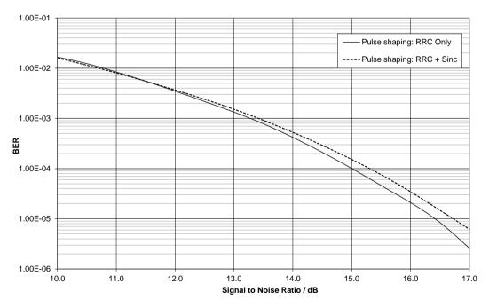
Figure 43 12.5kHz Channel Sensitivity With and Without Sinc Filter Comparison
